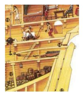
The Whiplash (15), a steering pole with a gimbal turning ball, attached to (14) the tiller, attached to the rudder (13)
