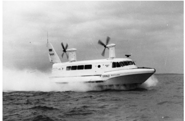
The SR-N2 at speed, achieving 80 knots on calm waters and holding 75 passengers
